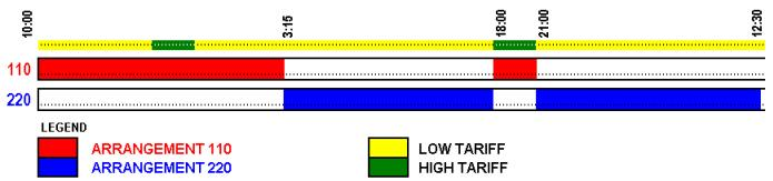
Figure 7: Optimal distribution of pumping arrangements – Case Study 1
