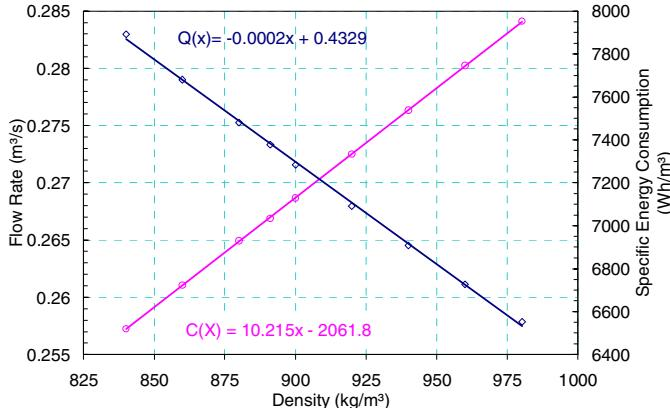
Figure 6 – Density influence on the maximum flow rate and minimum specific energy consumption. Pumping arrangement 2+2+0.
