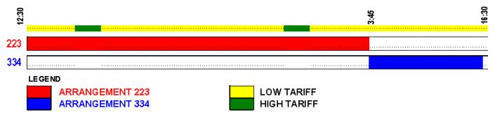
Figure 8: Optimal distribution of pumping arrangements – Case Study 2
