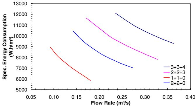
Figure 4 – Pump specific energy consumption as a function of flow rate.
