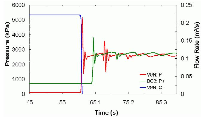
Figure 2.b. Pressure transient at check and block valves for an instantaneous closure (1 second) of block valve (V9N).
