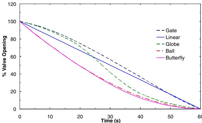
Figure 6. Closing curve of the block valve V9N.
