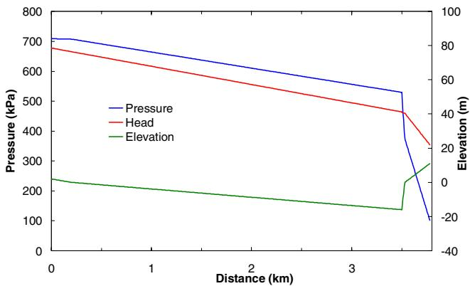
Figure 3. Pressure, head and elevation profiles at steady state.
