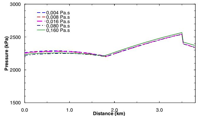
Figure 15. Maximum pressure profile for different viscosities maintaining the density constant.
