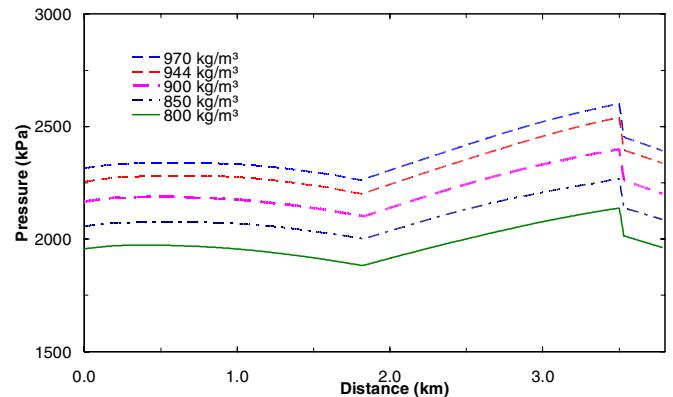
Figure 14. Influence of fluid density on the maximum pressure profile. Viscosity kept constant.
