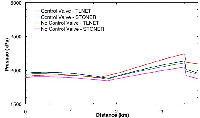
Figure 4. Maximum pressure profile for 60-second valve closure time. Results from SPS and TLNET with and without a flow control system.
