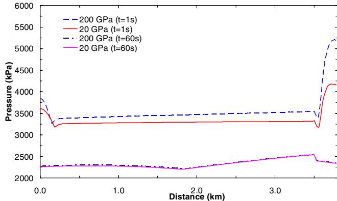
Figure 13. Influence of flexible pipe modulus of elasticity on maximum pressure profile
