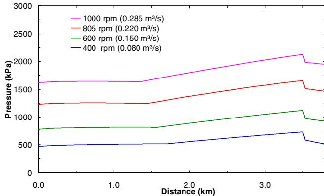
Figure 9. Maximum pressure profile for different flow rates obtained by the variation of pump rotation.
