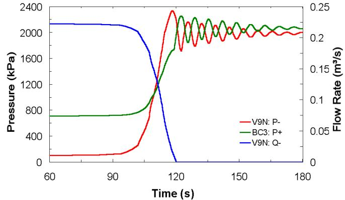
Figure 2a. Pressure transient at check and block valves for a 60-second closure time of the block valve (V9N).
