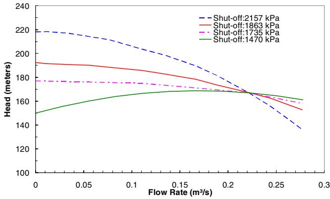
Figure 10. Modified pump curves with the same point of operation.
