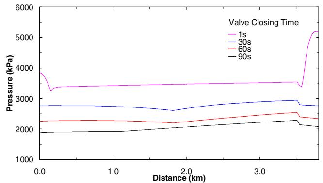
Figure 5. Maximum pressure profile for different valve closing times.
