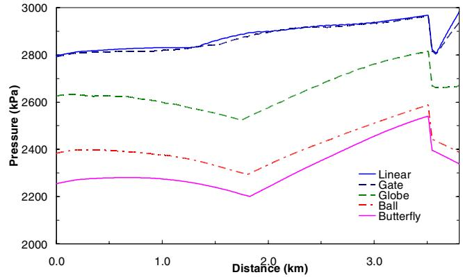
Figure 7. Maximum pressure profile for different types of block valves.
