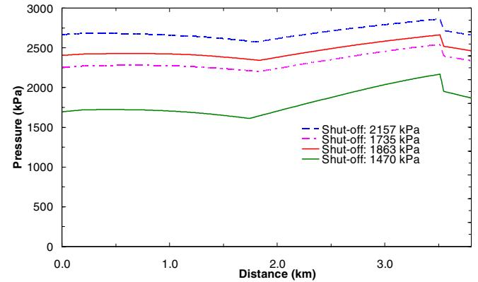
Figure 11. Maximum pressure profile generated by modified pump curves. Influence of shut-off value.
