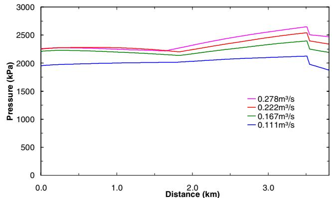
Figure 8. Maximum pressure profile for different flows regulated by flow control valve (PCV)
