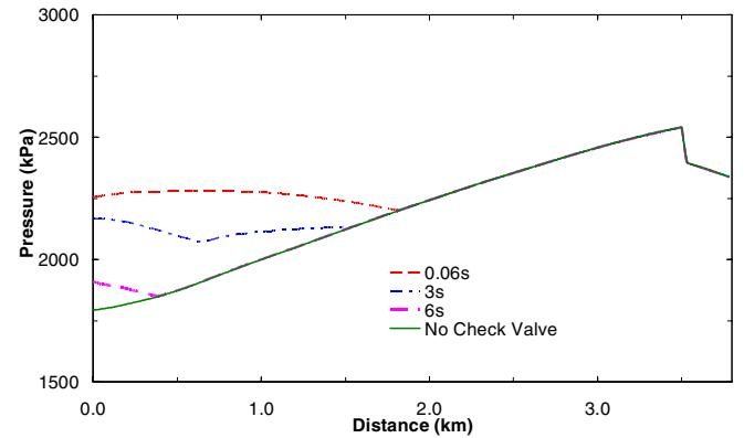
Figure 12. Maximum pressure profile as a function of check valve closing time.
