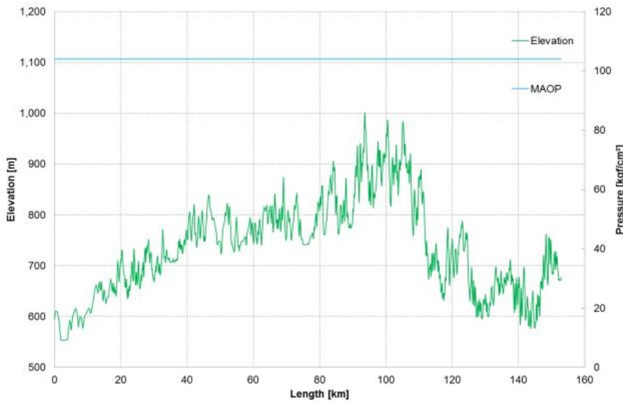
Figure 2, Pipeline profile and MAOP
